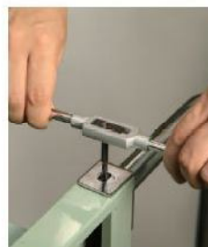
When hand tapping, always use tap wrench
